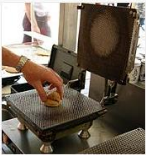
A ball of dough is placed on a waffle iron to make the waffle for a stroopwafel
